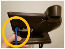
6. Plug the Power Injector into a wall outlet
