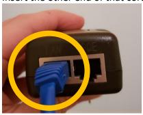
4. Take the other cord and insert one end into the Power Injector's POE port
